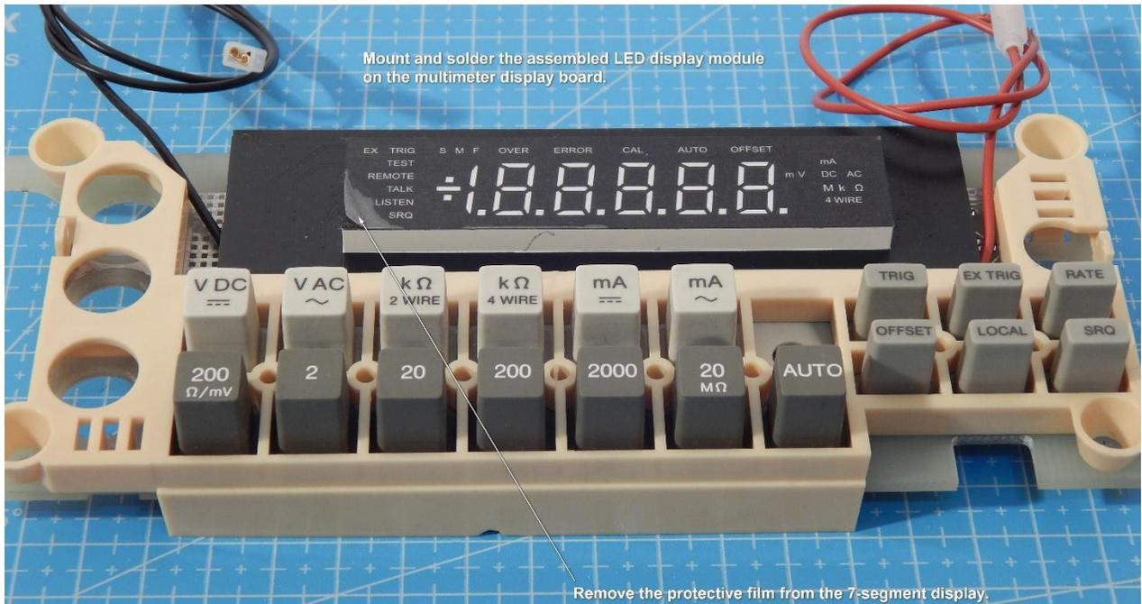
Remove the protective film from the 7-segment display.
